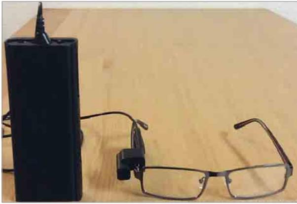
A. The OrCam unit, a miniature camera (on eyepiece of glasses), and a bone conduction earpiece (in front of ear) are mounted on the right side of a glasses frame. A cord connects the unit to a portable battery and computer pack. B. The OrCam unit connected to the battery and computer pack.
