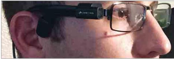
B OrCam unit connected to the battery and computer pack
